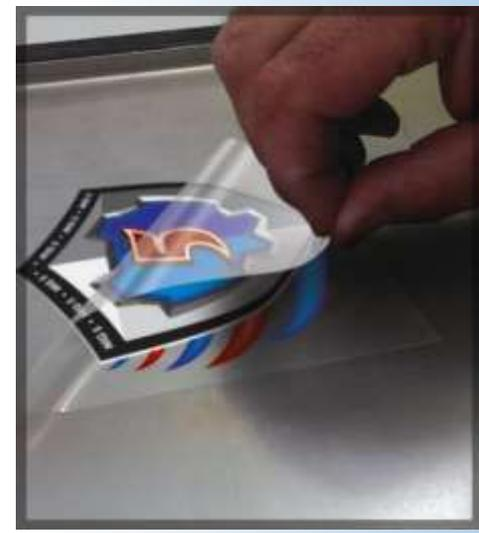
1. Position the Mold In Graphic in the mould – easy to slide into position
