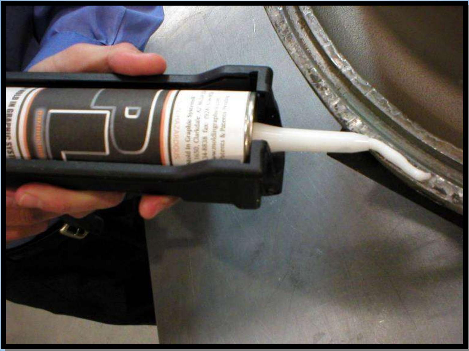
**Apply PL-S<sup>®</sup> directly to damaged areas of the parting line.**
