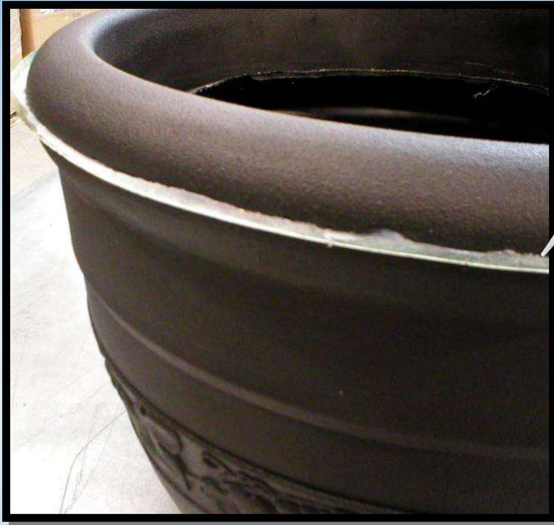
**PL-S<sup>®</sup> forms a solid bead which is easily removed by standard trimming operation.**
