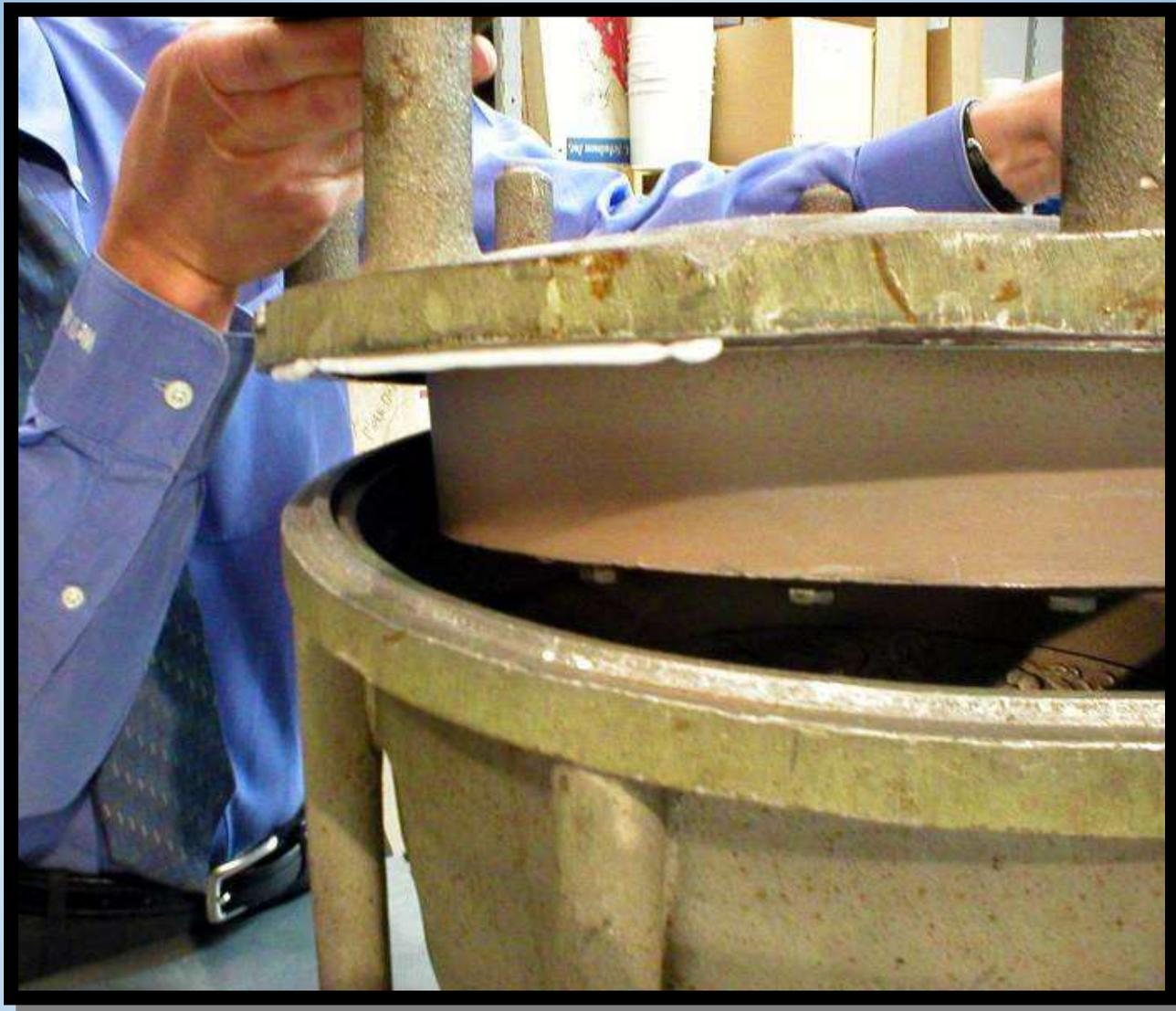
**After PL-S<sup>®</sup> is applied, close the mould per normal operating procedure.**
