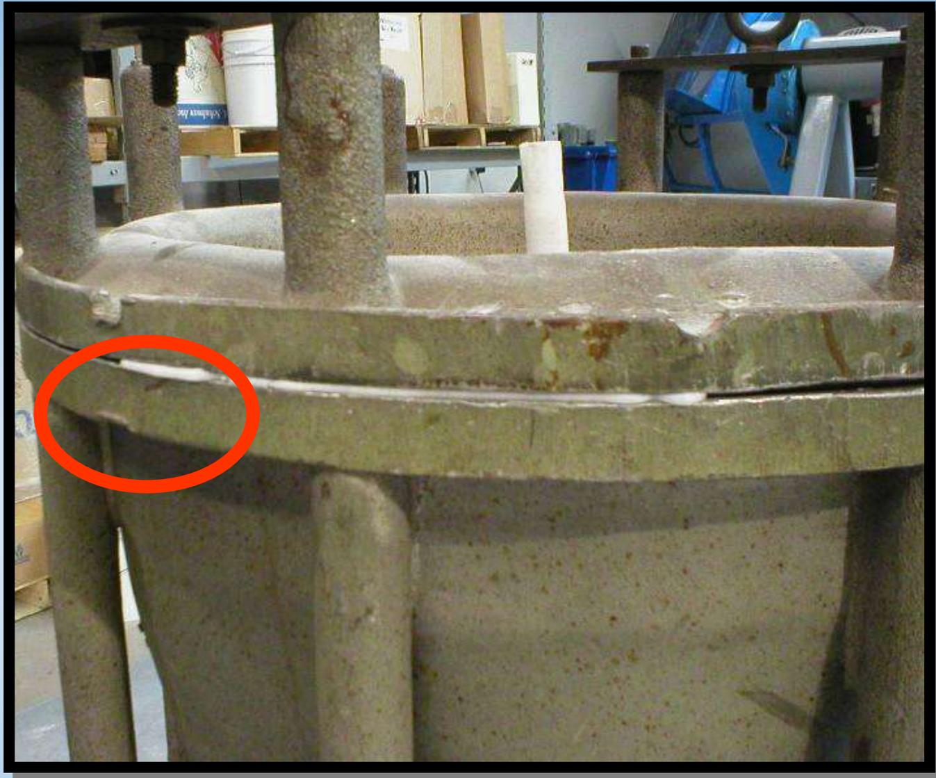
**PL-S<sup>®</sup> forms a complete seal at the parting line. This prevents escape or entrance of internal and external gases.**
